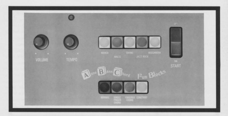
The BK-2 is equipped with a "Fun Block" section of four buttons which can be used in conjunction with the Auto Rhythm section (see p. 5). It enables you to play a variety of alternating bass chord rhythms, simply by holding down either a single lower manual key or a lower manual chord, according to which fun block button you press.
