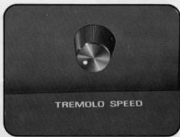
When the speed control is set to its maximum position, the Tremolo tablet will turn the speaker at seven revolutions per second. The Chorus tablet will turn it at one revolution per second.
