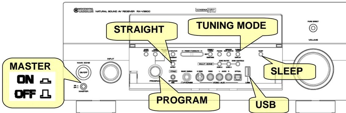
**Step 2.** Confirm that the AC power cable of the Yamaha receiver is plugged to the wall outlet and [MASTER] button is switched to the OFF position.
