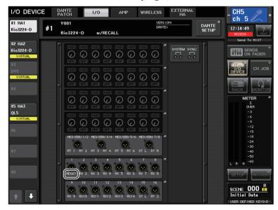
When the CL/QL console is in AES67 mode, the settings for the following parameters cannot be changed on the console.
