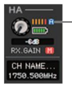
The RF channel (A or B) display has the same design as for the AXT400.
