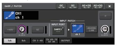
Press the INPUT PORT button, and on the PORT SELECT window select the port to which the output signal from the AXT400 is connected (OMNI 1).
