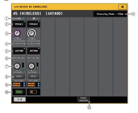
1 This indicator lights up when there is a connection via a ShowLink® remote control.
