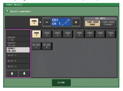
This assigns the output signal from the AXT400 to the input channel, and at the same time allows you to control and monitor the level of the AXT400 from the input channel.
