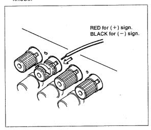
2. Banana Chip connections are also possible. Simply insert the Banana Chip connector into the corresponding terminal.
